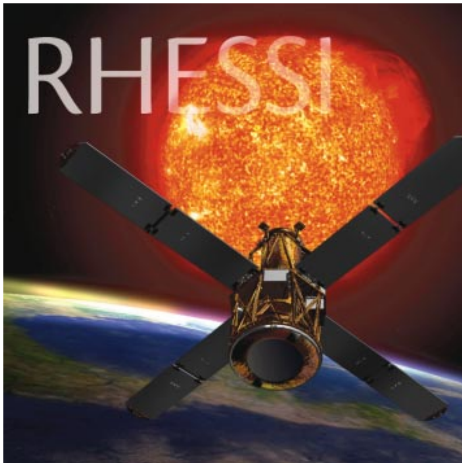
In this illustration the RHESSI X-ray telescope flies at 373 miles above Earth, using the Earth's magnetic field to align itself with the sun. RHESSI rotates about its axis once every four seconds and uses this rotation as part of an ingenious imaging system to capture X-ray images of solar flares.
