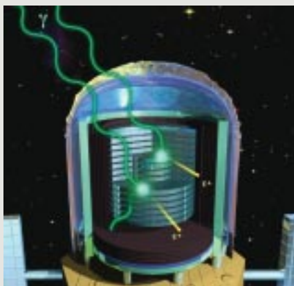
Inside TIGRE, gamma rays impacts produce positrons that are tracked through several detector layers to determine their direction.
